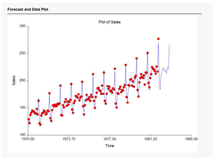
The data plot lets you analyze how closely the forecasts track the data. The plot also shows the forecasts at the end of the data series.
