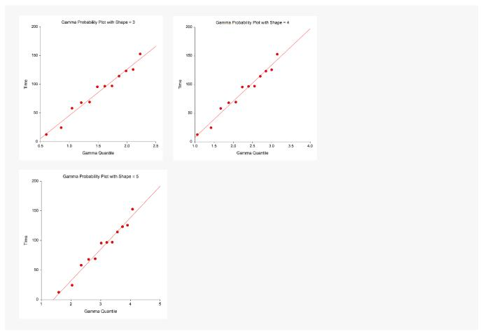
There is a gamma probability plot for each specified value of the shape parameter (set in the Prob.Plot Shape Values option of the Search tab). The expected quantile of the theoretical distribution is plotted on the horizontal axis. The time value is plotted on the vertical axis. Note that censored points are not shown on this plot. Also note that for grouped data, only one point is shown for each group.
