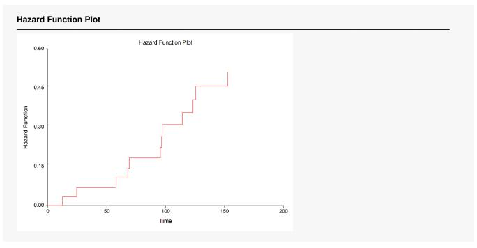
This plot shows the cumulative hazard function for the data analyzed. If you have several groups, then a separate line is drawn for each group. The shape of the hazard function is often used to determine an appropriate survival distribution.
