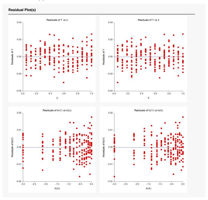
These are scatter plots of the residuals versus each of the independent variables. Note that some of these plots show the data in the transformed (In(Y), In(U), and In(X)) scale.
