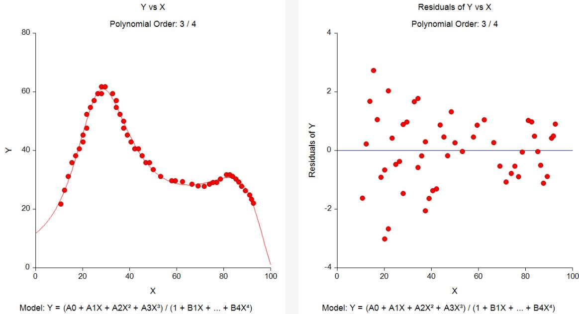
These plots show a plot of the data with the model fit overlayed on the left and the residuals on the right. These plots will allow you to detect any unwanted characteristics in this model. Note that none can be seen in these plots.
