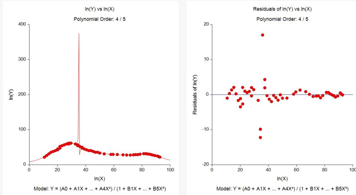
These plots show a problem that can occur with ratio of polynomial models. The strange plot occurs because the denominator polynomial includes a value near zero when  $X$  is just below 40. Since the model divides by this close to zero amount, the function value increases towards infinity. This problem may also be seen in the residual plot on the right. Note that the model seems to perform very well with a pseudo- $R^2$  of 0.978. The only remedy is to discard this model.
