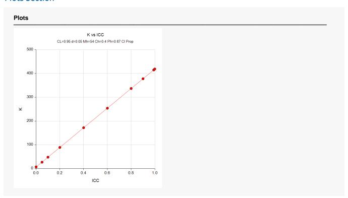
This plot shows the impact on sample size (number of clusters) of increasing *ICC*. The value of *K* increases from 7 to 419 and the value of N increases from 380 to 22,630.
