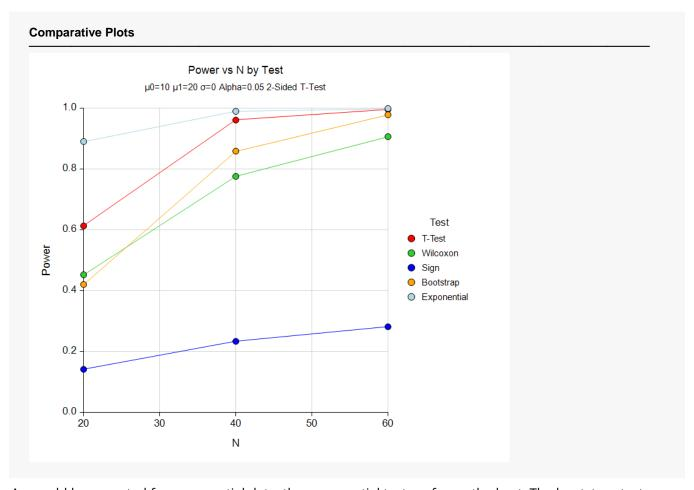
As would be expected for exponential data, the exponential test performs the best. The bootstrap test performs nearly as well for larger sample sizes. The other tests fail to achieve the target alpha level. Note that these simulation results will vary from run to run because the samples generated are random. The researcher must now decide which test to use based on her level of confidence in the data being truly exponentially distributed and the size of a sample she can afford to take.
