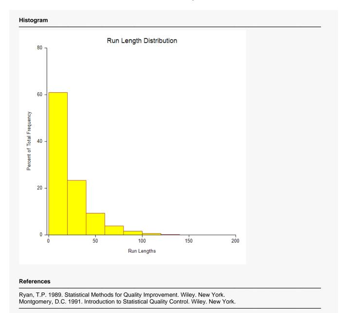
The results will vary slightly because they are based on simulation. The plot shows the distribution of run lengths of 5000 simulated runs.
