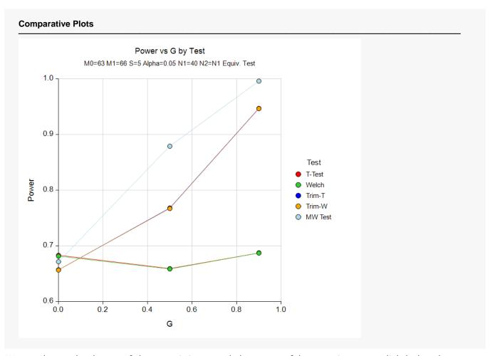
We see that as the degree of skewness is increased, the power of the t-test increases slightly, but the powers of the trimmed and nonparametric tests improve dramatically. The significance levels do not appear to be adversely impacted.
