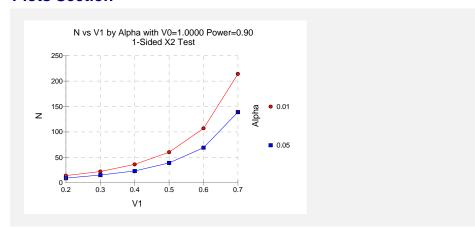
This plot shows the necessary sample size for various values of V1. Note that as V1 gets farther from zero, the required sample size increases.
