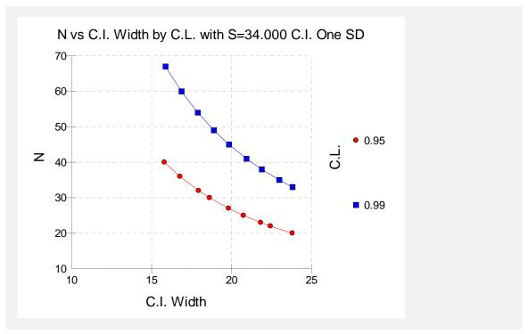
This plot shows the sample size versus the confidence interval width for the two confidence levels.
