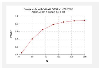
This plot shows the power versus the sample size. We see that a sample size of about 150 is necessary to achieve a power of 0.90.
