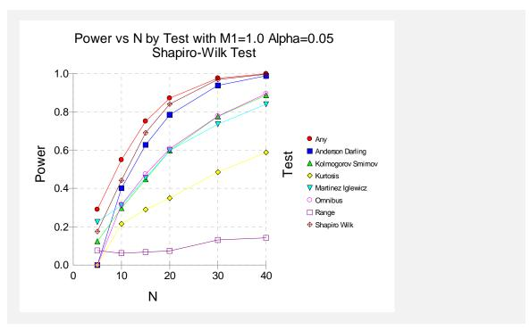
This plot shows performance of each of the normality tests. The champion is the Shapiro-Wilk test. The range test, which was designed for uniform alternatives, does very poorly with exponential alternatives.
