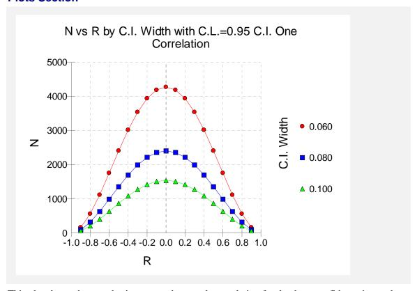
This plot shows the sample size versus the sample correlation for the three confidence interval widths.
