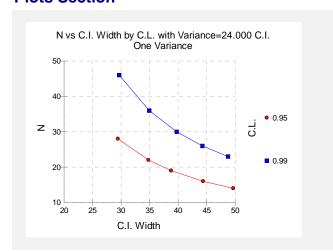
This plot shows the sample size vs. the confidence interval width for the two confidence levels.
