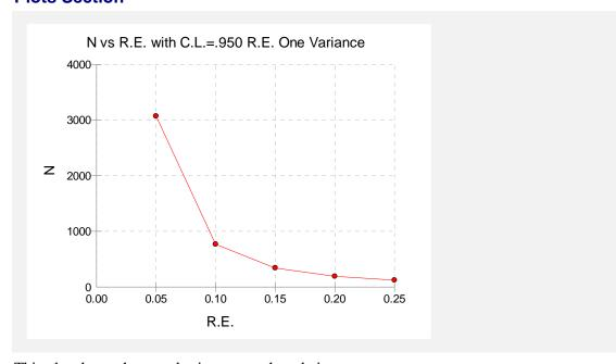
This plot shows the sample size versus the relative error.
