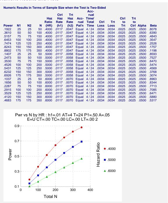
This plot shows the relationship between sample size and power for the three hazard ratios.
