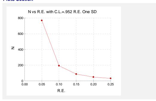
This plot shows the sample size versus the relative error.
