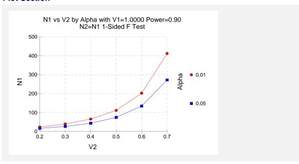
This plot shows the necessary sample size for various values of V2. Note that as V2 nears V1, the sample size is increased.
